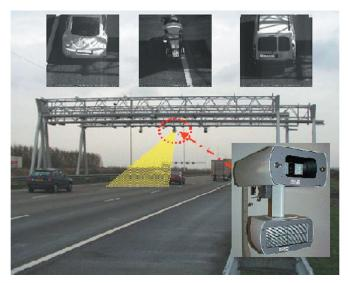
Vehicle Detection and Classification System. The system consists of a Detection computer placed in the cabinet and a set of gantry mounted laser scanners.
