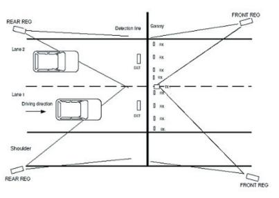
the detection system, and hence needs to be matched based on time comparison between the detection and communication system besides the lateral position information of the both the OBU and the vehicle.
